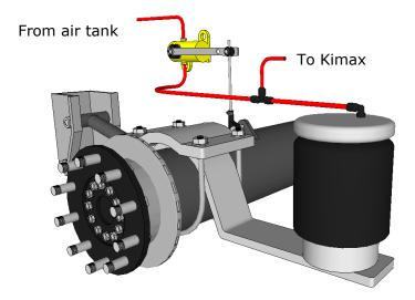
The pressure in the suspension system represents the weight of the axle/axle group.
