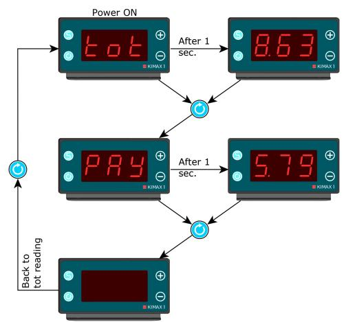
The Kimax instrument has a floating point. Values from 0.00 - 9.99 will be displayed with 2 digits after the decimal point. Values from 10.0 - 99.9 will be displayed with 1 digit after the decimal point. Values from 100 - 999 will be displayed without digits after the decimal point.
