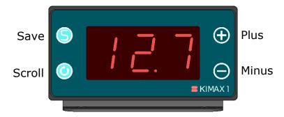
When the unit starts up it shows **tot** and after 1 sec. the display reads the value of the currently measured weight of your vehicle/axle/axle group.
