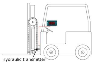
The hydraulic transmitter should be placed as close to the lifting cylinder as possible to obtain the best measuring accuracy.
