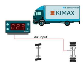
A dual air inlet channel is used on vehicles with split level control for one or more axles.
