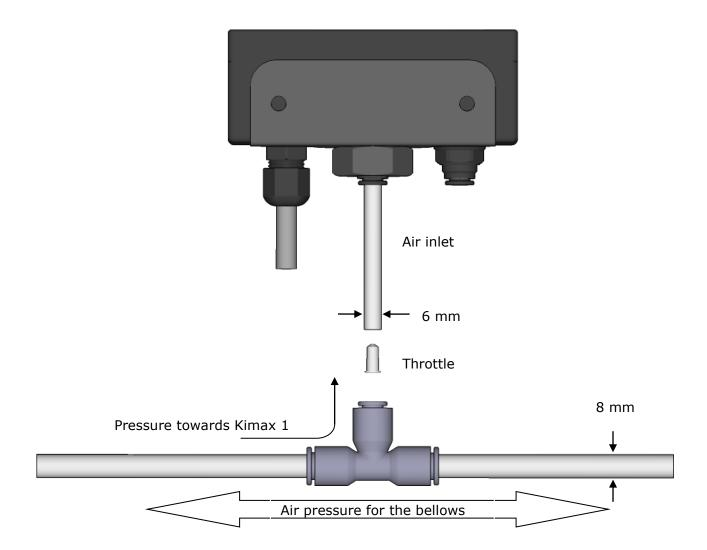
The Kimax instruments are equipped with push-in fittings.
