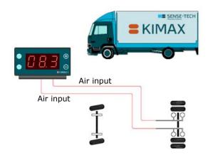
A dual air inlet can be applied on vehicles with one or more individual axles arranged in a combined level control system.
