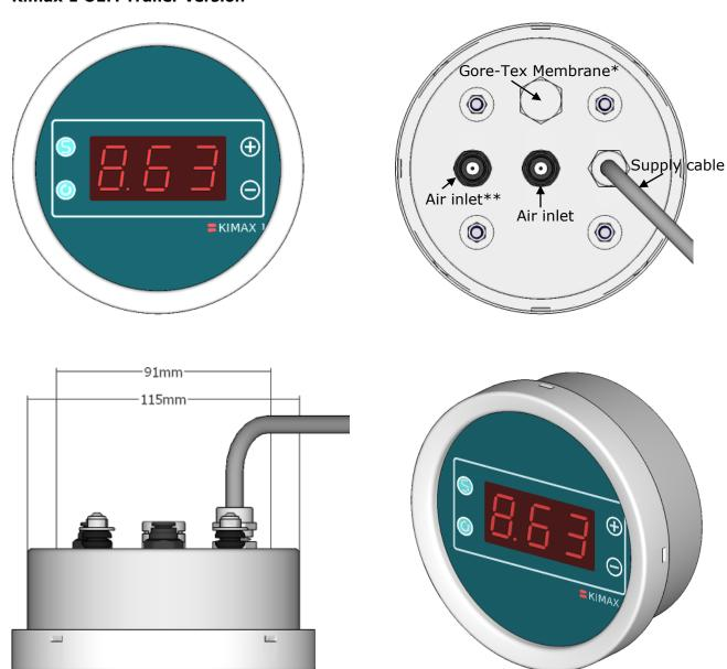
\*The Gore-Tex membrane is for venting the Kimax 1 housing, to avoid getting vacuum in the housing during shifting ambient temperatures.
