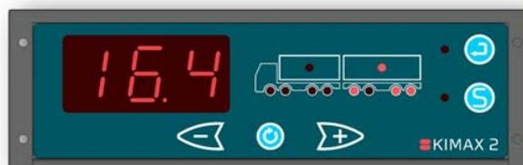
When you press
