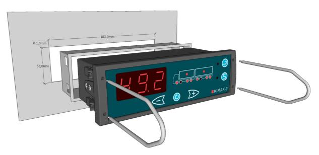
In order to replace the Kimax 2 Radio, you need to use the two belonging forks for releasing the snaps before you can pull the instrument out of the frame.
